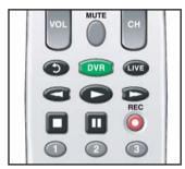
While in normal play mode, press **Rewind** or **Fast-Forward** to cycle through four different speeds of rewind or fast-forward.
