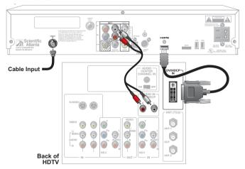
**Note**: When connecting the HDMI connector to the HDTV's DVI connector, you need an HDMI-to-DVI adaptor, and you need a separate audio connection.
